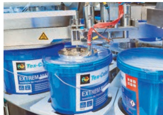
Leak test control of buckets sealed with peelable safety film
