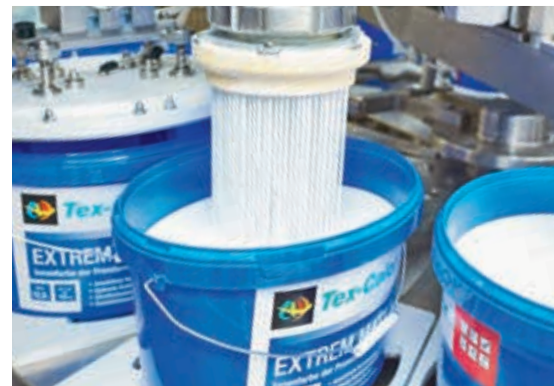
Filling station guaranteeing maximum dosing accuracy ( \leq 0.1\% standard deviation)
