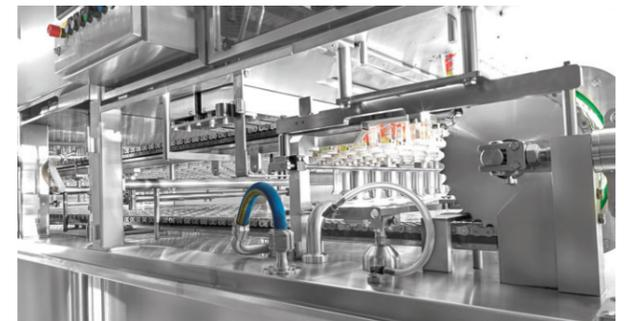
*Insight into high-performance filling machines: Rotary-type and linear cup filling machines in ultraclean design and with packaging material sterilisation  $\geq$  LOG 4*
