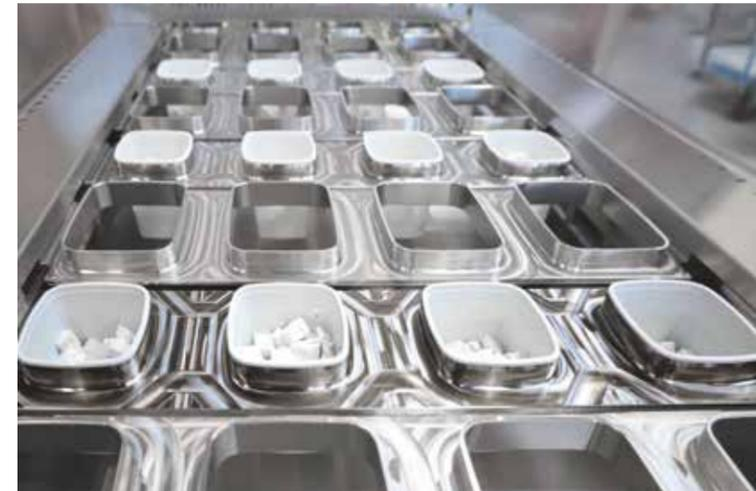
*View into a 4-lane cup filling and closing machine GRUNWALD-FOODLINER 6.000 in double-step design*
