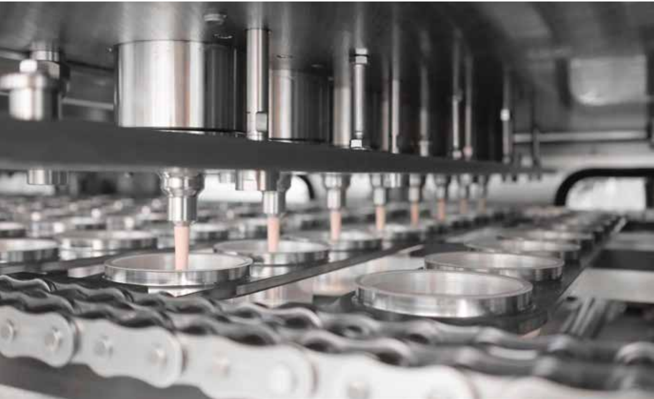
Filling of stirred yoghurt on the fully automatic cup filling and closing machine GRUNWALD-FOODLINER 20.000UC in 2x8-lane ultraclean design
