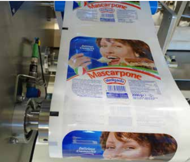
For guaranteeing maximum safety, the sealing film is sterilised by pulsating UV(C) high-performance radiators.
