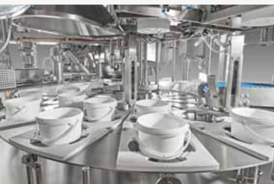
View into the 2-lane rotary table; it is designed for round and rectangular buckets
