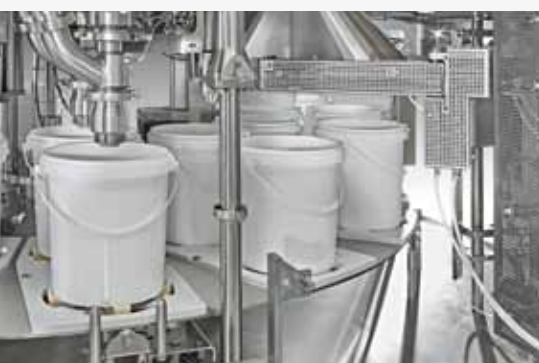
2-lane, weigh-controlled filling station
