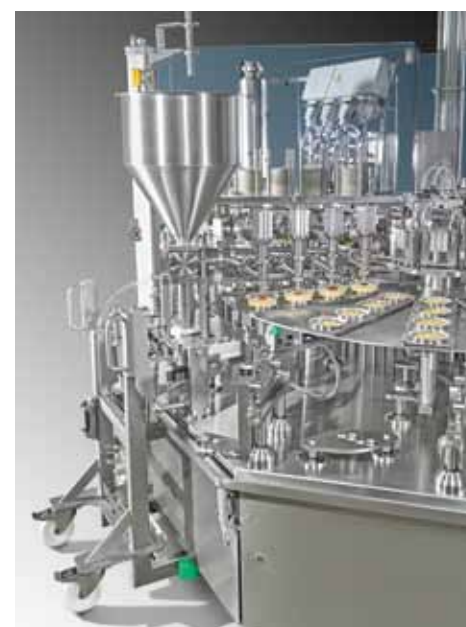
Partial view and overall view of 4-lane filling machine GRUNWALD-ROTARY 20.000
