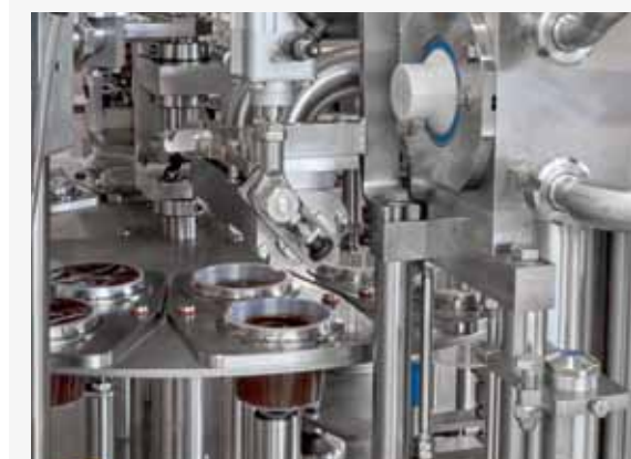
View of the rotary turntable on the rotary-type filling machine, filled with cups prior to the sealing process
