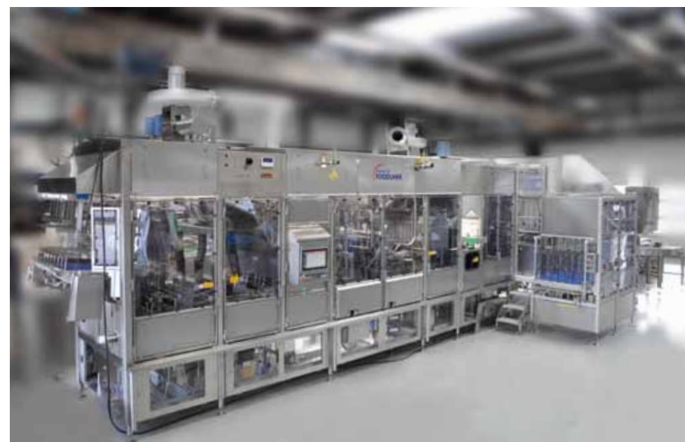
6-lane GRUNWALD-FOODLINER 12.000 cup filling machine in our plant in Wangen, shortly before delivery
