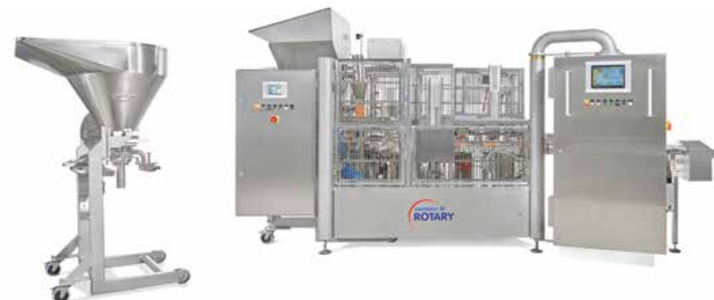
1-lane GRUNWALD-FLEXODOS for filling non-pumpable, free flowing products, connected to the dock-in station of a cup filling machine type GRUNWALD-ROTARY 12.000. Alternatively, a mobile piston filler type MOBIFILL for pumpable products can be connected at the same position in exchange for the FLEXODOS
