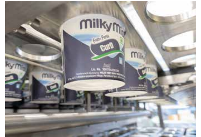
View into the 8-lane linear filling machine GRUNWALD-FOODLINER 20.000 while filling cups
