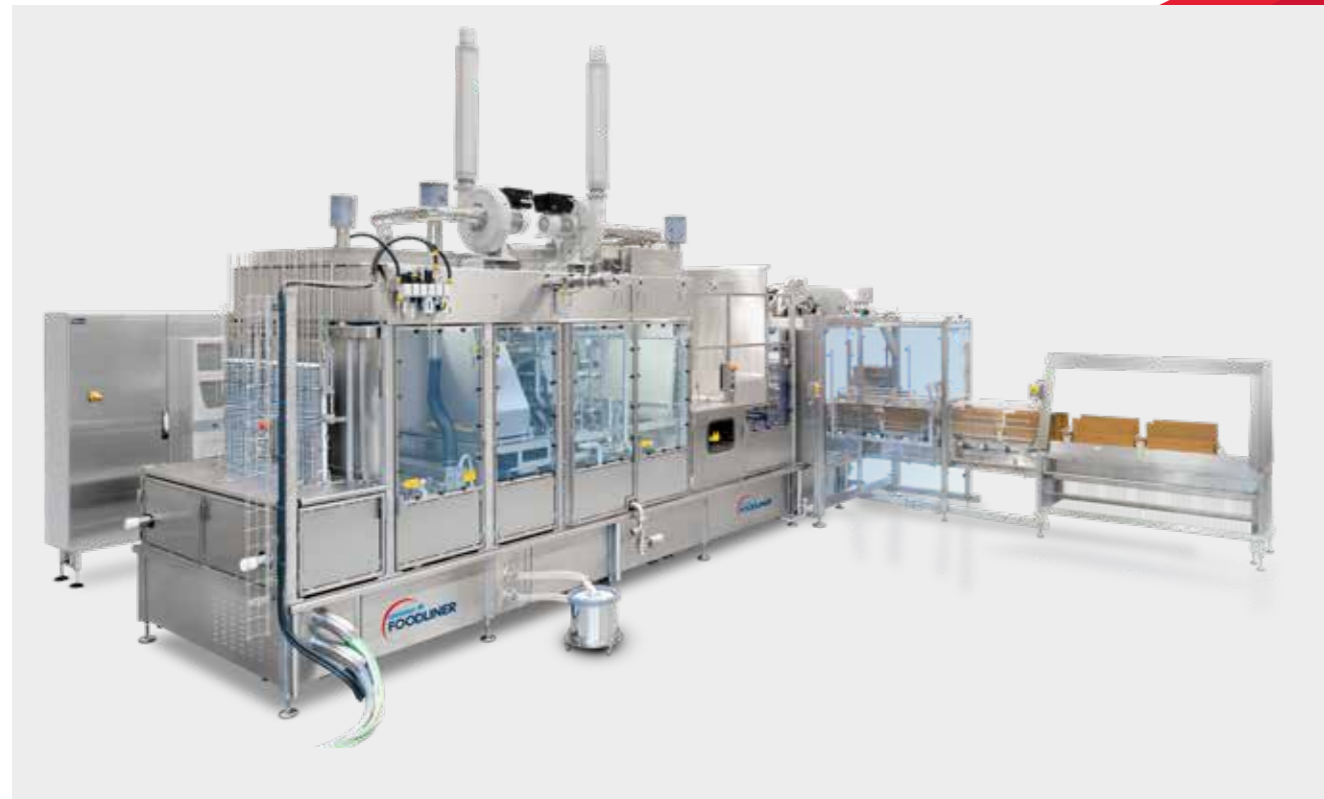
High-performance, 8-line cup filling machine GRUNWALD-FOODLINER 20.000 with integrated packer
