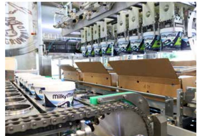
View into the 8-lane linear filling machine GRUNWALD-FOODLINER 20.000 while filling cups
